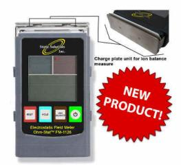
Item # Description FM-1126 Digital ESD Field Meter with Attachable Ionizer Plate
