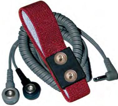
The adjustable WB2500 series features two 4mm snaps and 180 degree conductive paths around the wrist, providing maximum skin contact. The double snap coil cords provide two conductive paths to ground. Used with dual wire constant monitors.
