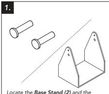
Line up the top holes in the Base Stand (2) and the Dispenser Box (1) and screw in the two supplied Screws (3.1 & 3.2) two supplied Screws (3.1 & 3.2)
