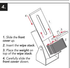
\*Carefully place the weight and slide down the front cover to avoid damage to base
