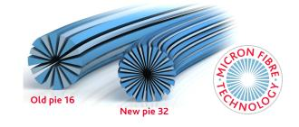
The size of a microfiber is 1 dTex (10 000 meter fiber per gram) or 50 times thinner than a hair. Today development has gone further and we are down in microfilament in size.
