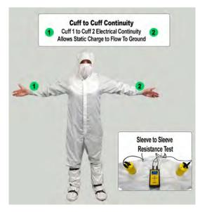
is made with a reliable ISO 6 static dissipative fabric with each component hood, coverall, boots—connected with conductive thread and ground snaps. Conductive boot soles eliminate static from personnel through the cleanroom ESD floor or mat. The garments system's superior workmanship and reliable panel-to-panel continuity makes it compliant with IEST-RP-CC052 and ANSI ESDS.2020 standards. The TX4000 Garment System maintains consistent continuity readings for up to 100 wash cycles.
