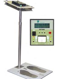
The OHM Metrics<sup>™</sup> PDT800K is a comprehensive, accurate ESD Ground Device Tester that fully meets your daily ESD checking needs. The PDT800K independently tests the left and right foot and wrist band and gives a visual and audible PASS/FAIL indica-tor. An innovative LCD screen will instantly display the test result and the measured resistances so you can easily understand your testing program.
