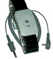
Dual Wire Wrist Straps provide redundancy; even if one dual wire wrist strap conductor is severed, the operator has reliable path-to-ground with other wire. The expandable metal band features a single mono jack fastener capable of reading both sides of the wrist strap. Used with dual wire constant monitors.
