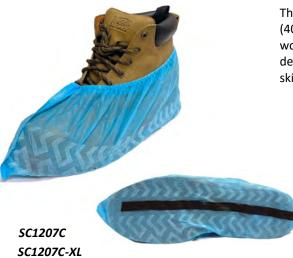
The ESD shoe covers are made from two (2) pieces of heavy-weight 1.25oz (40 gm) polypropylene and work well as a stand alone shoe cover or when worn inside laundered boot covers. The surged-seam inside shoe cover design features an elastic opening that fits most regular shoe styles. A non-skid coated soles provide better traction and improved safety.
